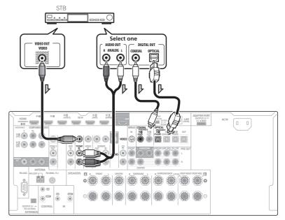
If your set-top box is equipped with an HDMI output terminal, we recommend connecting it to the receiver's HDMI IN 1 or IN 2 terminal. When doing so, also connect the receiver and TV by HDMI (see *Connecting using HDMI* on page 17).
